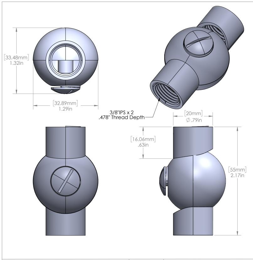
3/8" IPS x 3/8" IPS Friction Swivel 2.5 Lbs Max Load Available in White, Black, Nickel .478" Thread Depth Each End This Document
