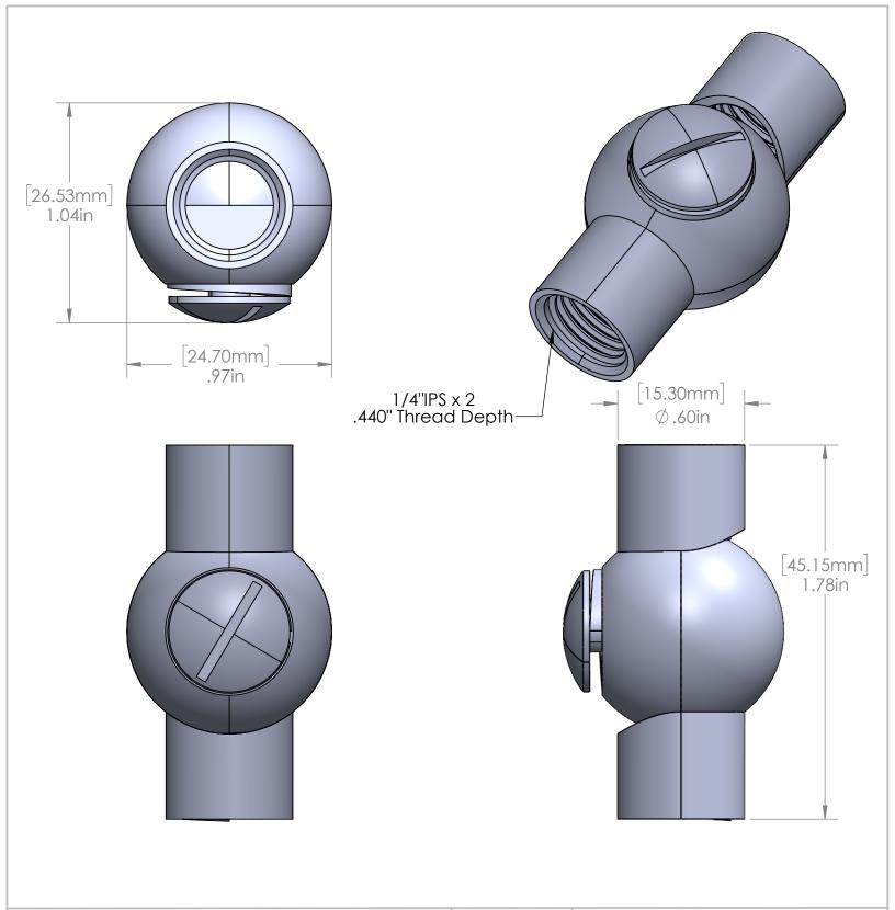
1/4" IPS x 1/4" IPS Friction Swivel 2.5 Lbs Max Load Available in White, Black, Nickel .440" Thread Depth Each End This Document
