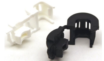
171 WHT/BK 7/8"(.875") KO Strain Relief for 18/3, 18/4 & 18/5 SJT Cord Connector Snaps and Locks around Cord Fits .290"-.385" cord
