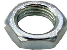
#64 Hex Nut 1/4"IP x 3/4"OD x 1/4" Thick Zinc Plated
