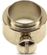
#12-.625" -1/4"IP Slip Ring #12-.625 for 1/4" IPS Stems Slip Ring .725" OD x .433" x .518" ID x .092" Flange for .625"Hole Mounting Zinc Casting w/8/32" Set screw
