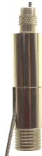
GR-SE 1/4IP Combo Side Exit Gripper for 3/32" Cable W/ Safety Nut 1/4"-20 Female & 1/4" IP OD on Bottom 3/32" Cable .513" x 2.05" Body 2.5" Overall HT. .25" & .5" Mounting Slots
