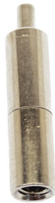
MGR CC 1/4-20 M Bottom Exit Gripper for 1/16" Cable .250" Mounting Hole 1.587"L x .345"W x .590" 1/4"-20 Thread
