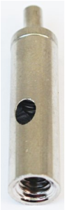
MGR-SE 1/4-20-M Side Exit Gripper for 1/16" Ca- ble. 1/4"-20 Female on Bottom. 0.250" Mounting Hole .237" Thread Diameter 1.667"H x 0.36" W x 0.425" Thread Depth
