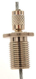
MGR-1/8IP Bottom Exit Gripper W/Safety Nut for 1/16" Cable 1/8" IP Male on Bottom .400" Mounting Hole 1.06"H x .589"W x .615" Thread
