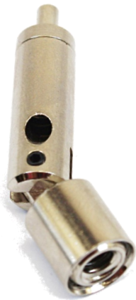
MGR-SE-360 1/4-20 LN Side Exit Gripper for 1/16" & 3/64" Cable W/Adjustable Foot (Moves in all Directions) .250" Mounting Hole 2.531" L x .467" W x .40625" Thread Length
