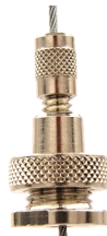
GR1/4IP-TN Bottom Exit Gripper W/Safety Nut & Top Nut for 1/16" & 3/32" Cable .562" Mounting Hole 1.25"H x .757"W x .2" Thread
