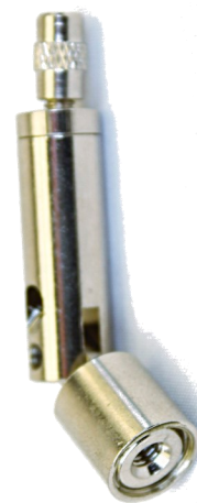
MGR-SE-360 8/32 Side Exit Gripper W/Safety Nut for 1/16" & 3/64" Cable W/ Adjustable Foot (Moves in all Directions) .187" Mounting Hole 2.531" L x .467" W x .40625" Thread Length
