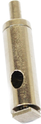
MGR-SE 8/32 SH Side Exit Gripper for 1/16" Cable 8/32" Female on Bottom 0.187" Mounting Hole .155" Thread Diameter 1.48"H (Top of Plunger)x 0.353" W x 0.25"D 8/32" Tapped Hole x 1.14" Body Length 0.200" Length of Screw Thread Screw head .265" x .310" High
