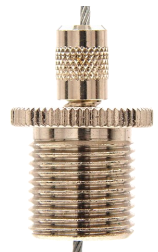
GR3/8IP Bottom Exit Gripper W/Safety Nut for 1/16" & 3/32" Cables 3/8" IP Male on Bottom .687" Mounting Hole 1.3"H x .885"W x .670" Thread
