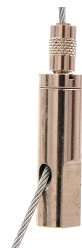
MGR-SE-1/4-20 Side Exit Gripper W/Safety Nut For 1/16" Cable 1/4"-20 Female on Bottom .250" Mounting Hole 1.653"H x .39"W x .235" Thread
