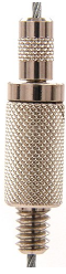
MGR-1/4-20 Bottom Exit Gripper W/Safety Nut for 1/16" Cable 1/4"-20 Male on Bottom .250" Mounting Hole 1.64"H x .4"W x .45" Thread
