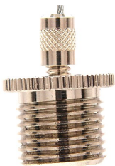
GR1/2IP Bottom Exit Gripper W/Safety Nut for 1/16" & 3/32" Cable 1/2" IP Male on Bottom .875" Mounting Hole 1.319"H x 1"W x .669" Thread
