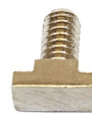
SLOT SCREW 1/4-20 1/4"-20 Threaded Screw w/T- Slot Head used to capture slotted extrusion .420" H x .450" L x .300" W .265" Thread Length
