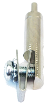
LG-32 Used w/ 3/32" cable (25-120 lbs working load). 2 slots for entrance and exit of cable on each side to form loops. Releasable without tools. .795" L x .899" w x .491" Thick
