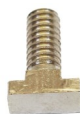
SLOT SCREW 8/32 8/32" Threaded Screw w/T- Slot Head used to capture slotted extrusion .420" H x .350" L x .180" W .285" Thread Length
