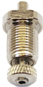
MGR 1/8 IP RG Reversing Mechanism Bottom Exit Gripper for 1/16" & 3/64" Cable .400" Mounting Hole .972"H x .512"W x .512"Thread
