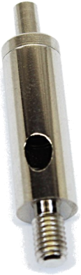
MGR-SE 10/32 EXT Side Exit Gripper for 1/16" Cable 1/4"-20 Male on Bottom .187" Mounting Hole 1.747"H x .351" W x .276" of 10/32" Thread
