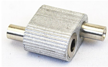
AL-LG 3/32 Aluminum Shot Blast Looping Gripper for 3/32" & 5/64" Cable .728" L x .893" W x .469" W 154 Lbs SWL for 3/32" Cable 123 Lbs SWL for 5/64" Cable
