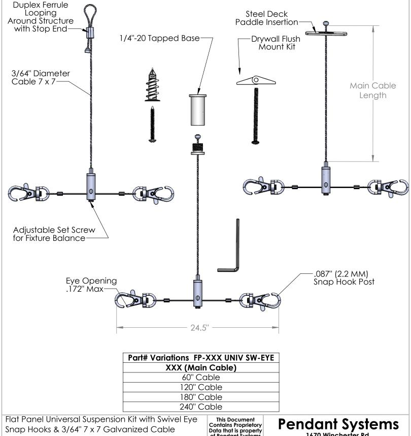
Flat Panel Universal Suspension Kit with Swivel Eye Snap Hooks & 3/64" 7 x 7 Galvanized Cable Applications: Drywall, Steel Deck & Loop Around Structure using Duplex Ferrule 2-Pack (Suffix-S Single Pack)Max Safe Static Load- 10 Lbs / Cable
