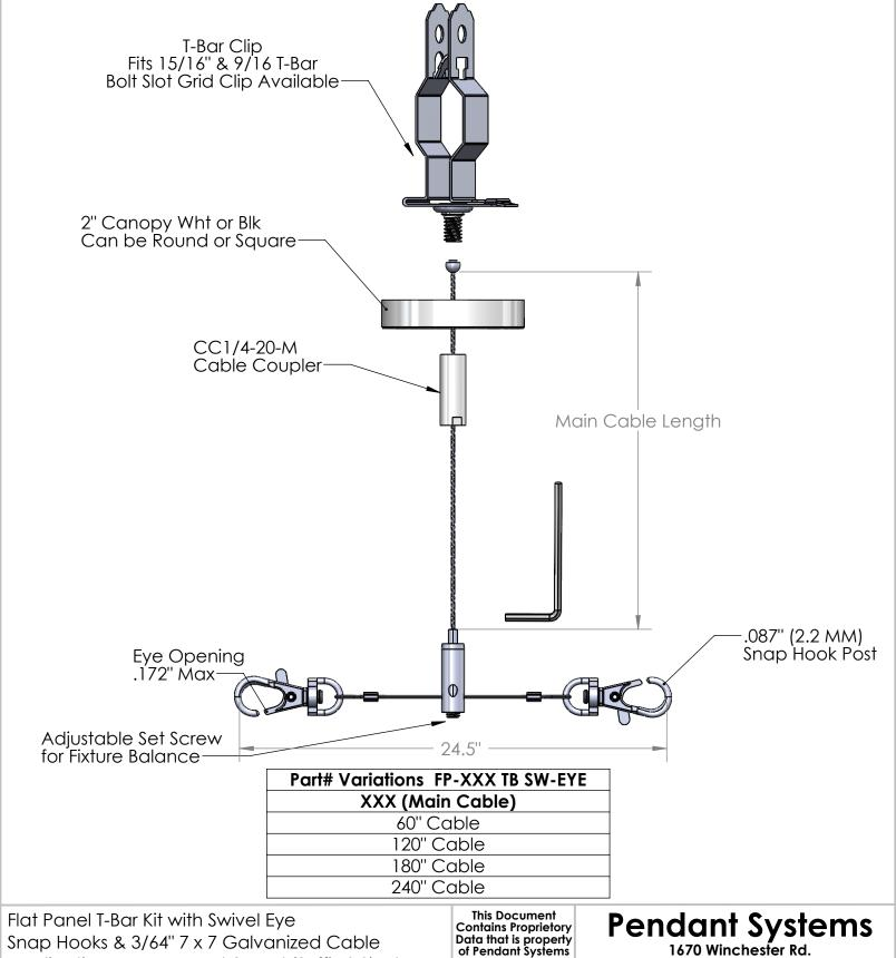
Flat Panel T-Bar Kit with Swivel Eye Snap Hooks & 3/64" 7 x 7 Galvanized Cable Applications: T-Bar Mount 2-Pack(Suffix-S Single Pack) Max Safe Static Load- 10 Lbs / Cable 10 Lb Fixture 5 X Safety Factor This Document
