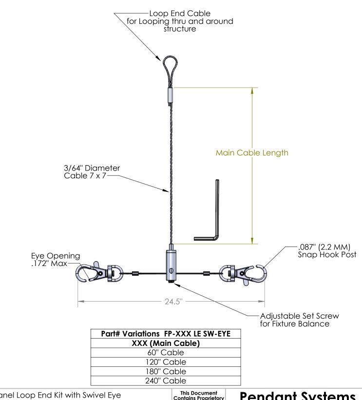
Flat Panel Loop End Kit with Swivel Eye Snap Hooks & 3/64" 7 x 7 Galvanized Cable Applications: Looping Mount 2-Pack(Suffix-S Single Pack) Max Safe Static Load- 10 Lbs / Cable 10 Lb Fixture 5 X Safety Factor
