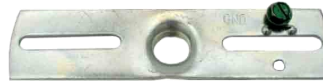
#39 Crossbar 1/4"IP Tapped Crossbar with Ground Screw Inserted 4 3/16"L x 1"W Zinc Plated x 14 Gauge
