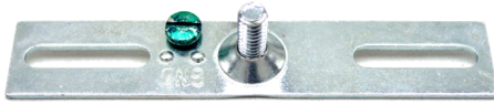
#158 Crossbar 1/4"-20 Countersunk Crossbar with Ground Screw & 1/4"-20 Flat Head Screw Inserted 3 7/8"L x 3/4"W Zinc Plated x 14 Gauge
