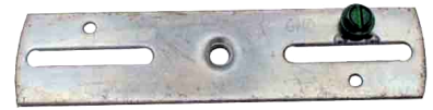
#108 Crossbar Heavy Duty 1/4"-20NC Bracket Crossbar with Ground Screw Inserted 4 3/16"L x 1"W x 14 Gauge Zinc Plated
