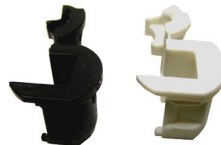
102BK 102 Lock-It Style Strain Relief for .625" PF Hole for 18/3 & 18/4 Fits .300"-.330" Cord Locks around cord before insertion
