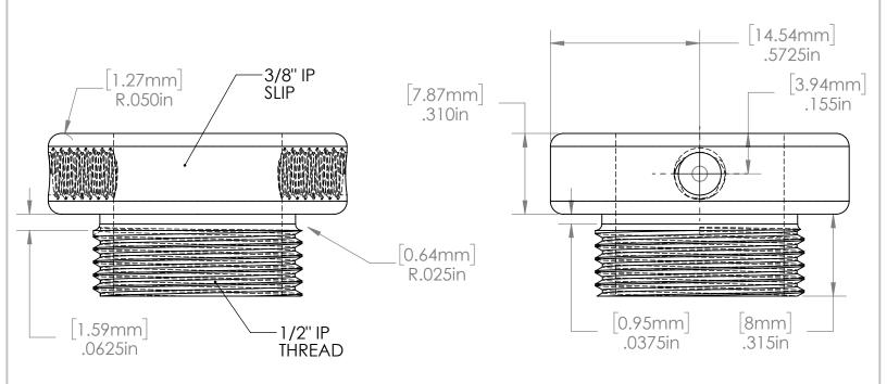
Stem Adapter for Field Cutting Stems without rethreading 1/2" IP Male x 3/8" IP Slip Female Fits .625" O.D. Tube (3/8" IP Size)
