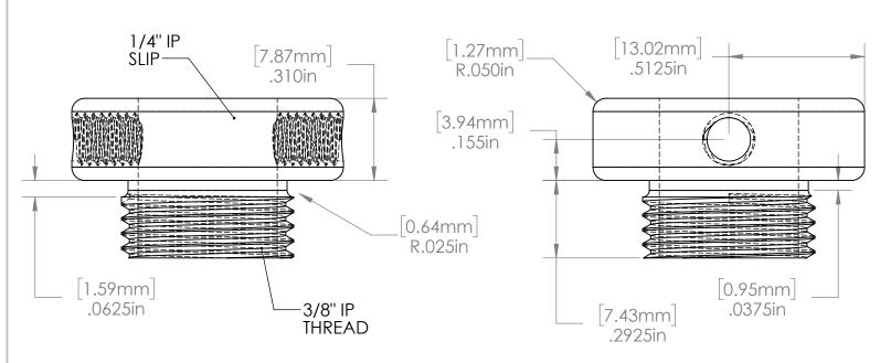
Micro Stem Adapter for Field Cutting Stems without rethreading 3/8" IP Male x 1/4" IP Slip Female Fits 1/2" O.D. Tube (1/4" IP Size)
