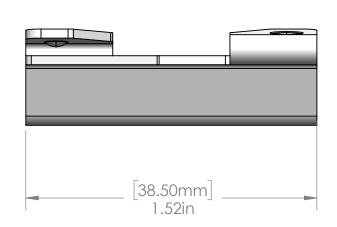
T-Bar Twist Clip for Acoustical T-Bar Ceiling Powder Coated White Fits Standard 15/16" T-Bar Accepts Half Ball end cables 1/32", 3/64", 1/16" 30 Lbs SWL This Document
