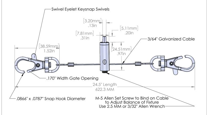
Micro-SE-TH W/24" Cable for Flat Panel Suspensions 3/64" Crosscable with Swivel Snap Eyelets Used with 3/64" & 1/32" Cables Max Safe Static Load - 10 Lbs / Cable 5 X Safety Factor
