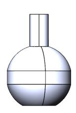
Micro Ball Gripper for 1/32" & 3/64" Cable Made for seating in .375" Hole Safe Static Working Loads 12 Lbs for 1/32" & 30 Lbs for 3/64" This Document
