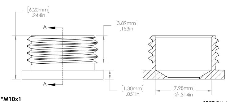
**THREAD** Used with AC1/16-[XXX] HB (#2 Diecast Half Ball End Stop) ONLY
