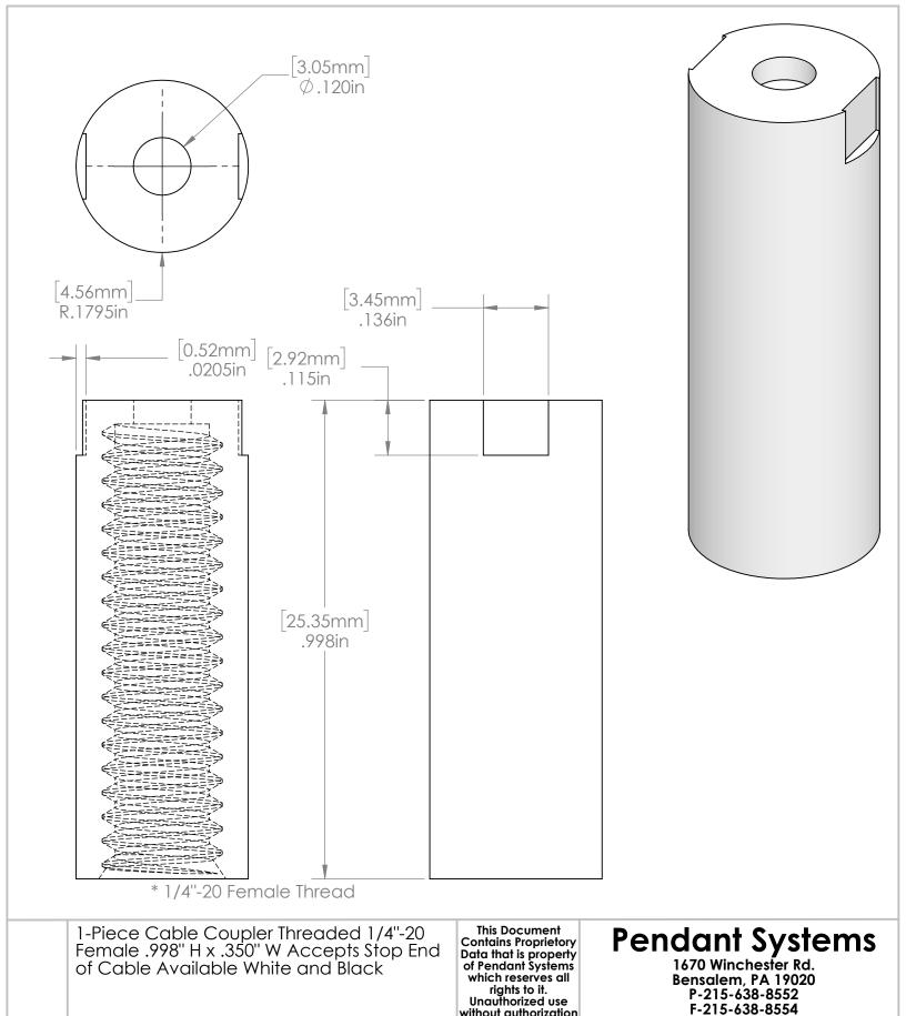
without authorization www.PendantSystems.com is prohibited. UNLESS OTHERWISE SPECIFIED DIMENSIONS ARE IN BOTH INCHES & FINISH: MILLIMETERS UNLESS OTHERWISE NOTED TOLERANCES: TITLE: CC1-4-20-M LINEAR: XX= .02" XXX= -.010" ANGULAR: + 1 Degree DO NOT SCALE DRAWING MATERIAL: Part # DEBUR AND BREAK SHARP EDGES REVISION SCALE: NTS SHEET 1 OF 1 DRAWN DATE: 3/10/16 Drawn By: MWR
