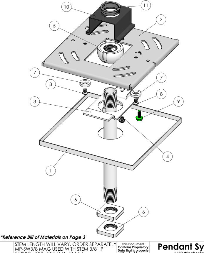
STEM LENGTH WILL VARY. ORDER SEPARATELY MP-SW3/8 MAG USED WITH STEM 3/8" IP 3/8" IPS .625"-.635" O.D. 18 T.P.I
