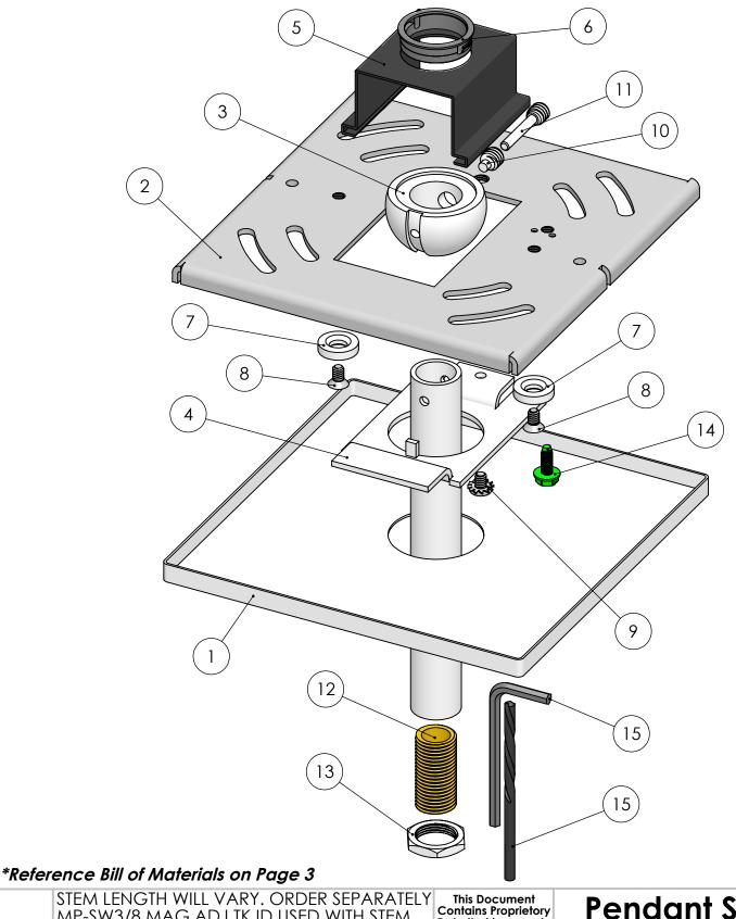
STEM LENGTH WILL VARY. ORDER SEPARATELY MP-SW3/8 MAG ADJ TK ID USED WITH STEM 3/8" IP I.D. PH 3/8" IPS .625"-.635" O.D. 18 T.P.I Add Suffix WHT for White or Bk for Black
