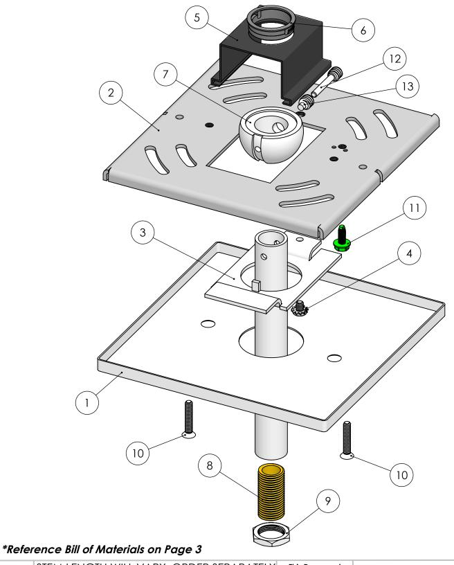
STEM LENGTH WILL VARY. ORDER SEPARATELY MP-SW3/8 ADJ ID USED WITH STEM 3/8" IP I.D. PH 3/8" IPS .625"-.635" O.D. 18 T.P.I
