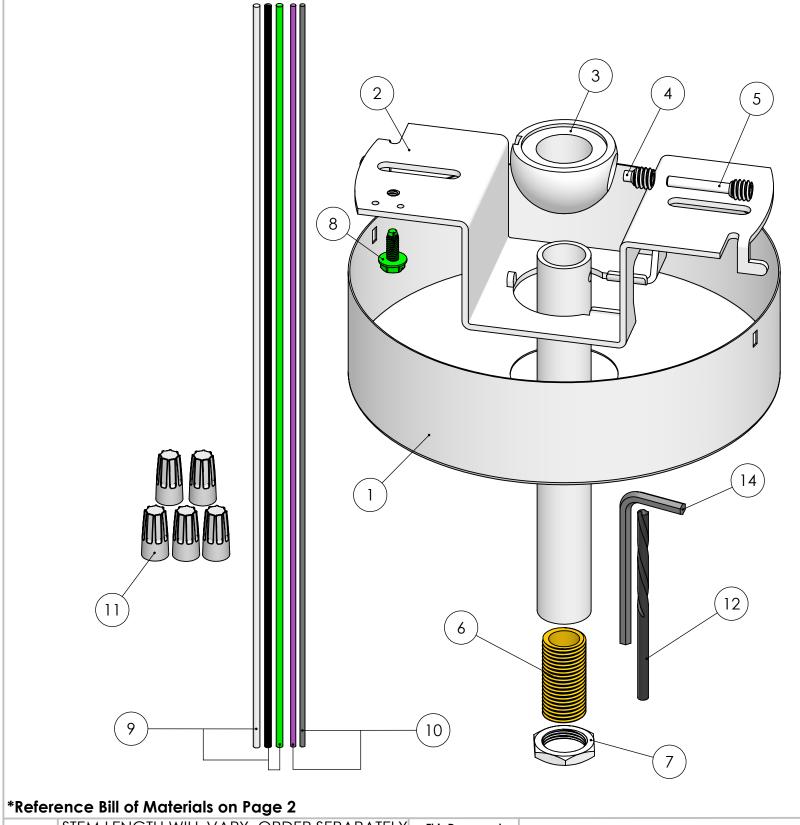
STEM LENGTH WILL VARY. ORDER SEPARATELY C545 TR ID ADJ TK 5W USED WITH STEM 3/8" IP I.D. PH 3/8" IPS .625"-.635" O.D. 18 T.P.I.
