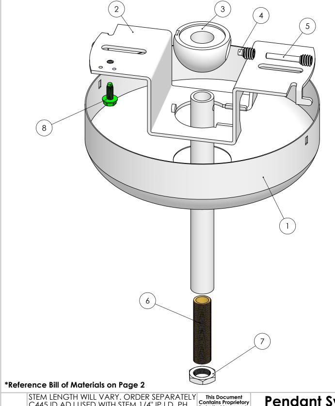
C445 ID ADJ USED WITH STEM 1/4" IP I.D. PH 1/4" IPS .500"-.510" O.D. 18 T.P.I.
