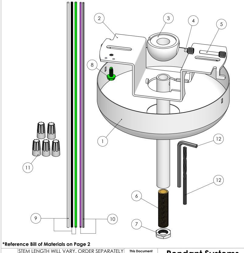
STEM LENGTH WILL VARY. ORDER SEPARATELY C445 ID ADJ TK 5W USED WITH STEM 1/4" IP I.D. PH 1/4" IPS .500"-.510" O.D. 18 T.P.I.
