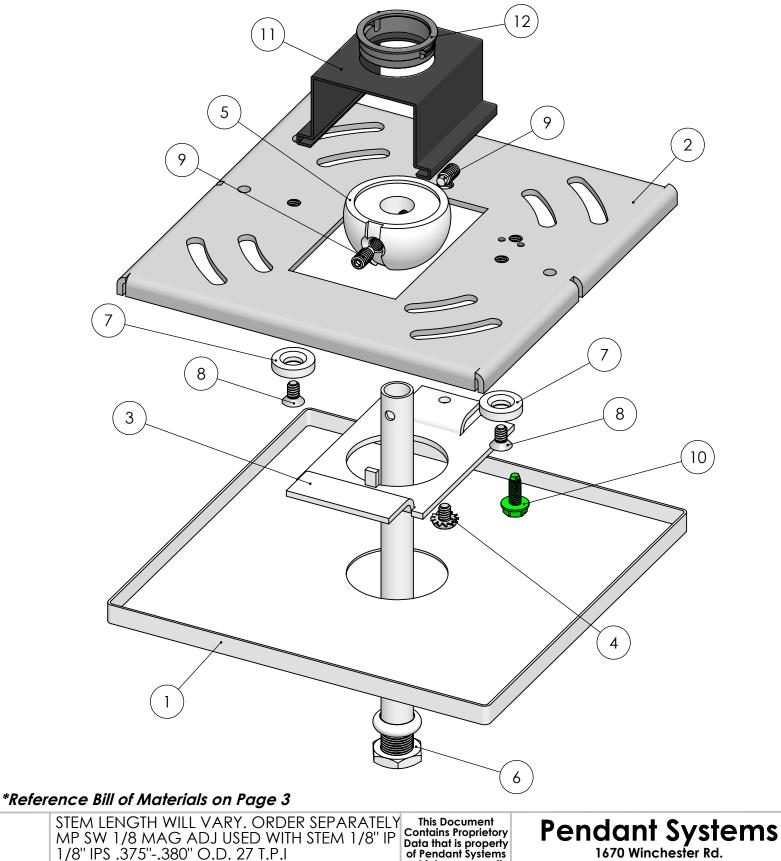
STEM LENGTH WILL VARY. ORDER SEPARATELY MP SW 1/8 MAG ADJ USED WITH STEM 1/8" IP 1/8" IPS .375"-.380" O.D. 27 T.P.I
