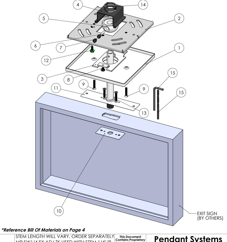
MP SW1/4 EX ADJ TK USED WITH STEM 1/4" IP O.D. PH 1/4" IPS .500"-.510" O.D. 18 T.P.I. Add Suffix WHT for White or Bk for Black
