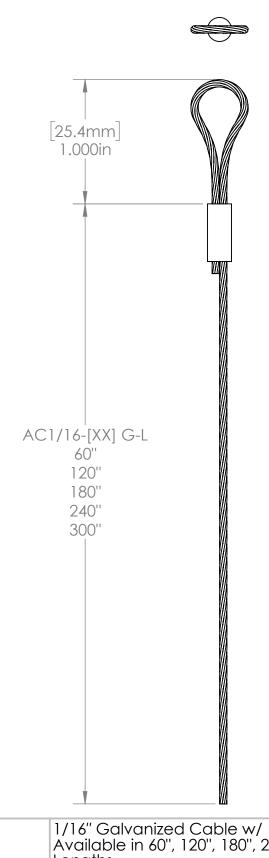
1/16" Galvanized Cable w/ 1" Loop Available in 60", 120", 180", 240" & 300" Lengths 7x7 Cable - MAX LOAD 480 lbs
