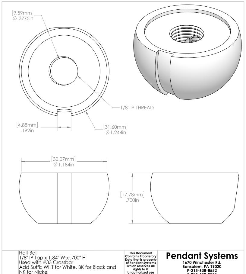
F-215-638-8554 without authorization is prohibited. www.PendantSystems.com UNLESS OTHERWISE SPECIFIED DIMENSIONS ARE IN BOTH INCHES & FINISH: MILLIMETERS UNLESS OTHERWISE NOTED TOLERANCES: TITLE: 1/8" IP Half Ball Bright Zinc LINEAR: XX= .02" XXX= -.010" ANGULAR: +1 Degree DO NOT SCALE DRAWING MATERIAL: Part # 272 DEBUR AND BREAK SHARP EDGES REVISION SCALE: NTS SHEET 1 OF 1 DRAWN DATE: 3/19/18 Drawn By: MWR
