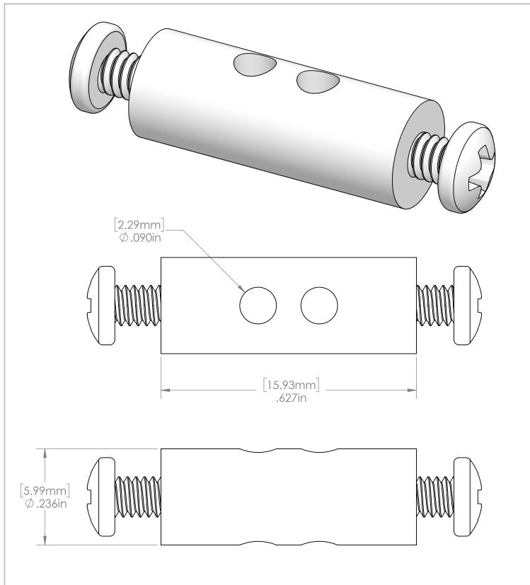
Cable Locking Tube .630" L x .236" W 2-Screws inserted at each end
