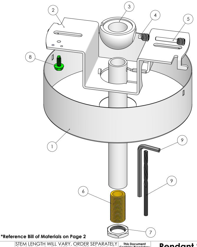
STEM LENGTH WILL VARY. ORDER SEPARATELY C545 TR ID ADJ TK USED WITH STEM 3/8" IP I.D. 3/8" IPS .625"-.635" O.D. 18 T.P.I.
