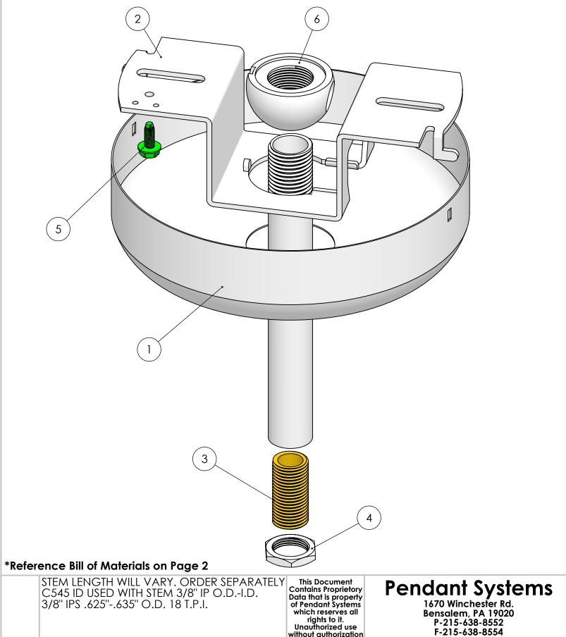
is prohibited. www.PendantSystems.com \*45° SWIVEL UNLESS OTHERWISE SPECIFIED DIMENSIONS ARE IN BOTH INCHES & MILLIMETERS UNLESS OTHERWISE NOTED TOLERANCES: TITLE: C545 ID LINEAR: XX= .02" XXX= -.010" ANGULAR: +1 Degree DO NOT SCALE DRAWING MATERIAL: Part # DEBUR AND BREAK SHARP EDGES REVISION SCALE: NTS SHEET 1 OF 2 DRAWN DATE: 9/11/17 Drawn By: MWR
