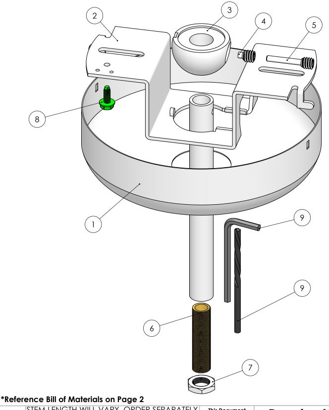
STEM LENGTH WILL VARY. ORDER SEPARATELY C445 ID ADJ TK USED WITH STEM 1/4" IP I.D. 1/4" IPS .500"-.510" O.D. 18 T.P.I.
