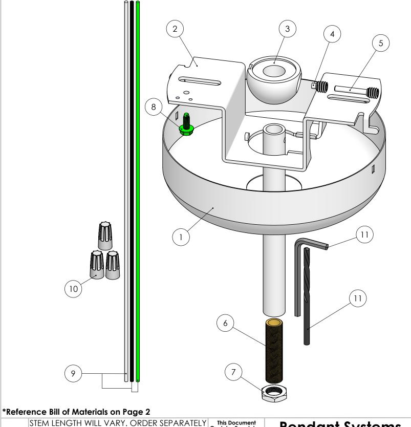
STEM LENGTH WILL VARY. ORDER SEPARATELY C445 ID ADJ TK 3W USED WITH STEM 1/4" IP I.D. PH 1/4" IPS .500"-.510" O.D. 18 T.P.I.
