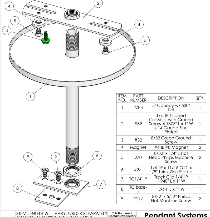
C415 TC MAG USED WITH STEM 1/4" IP 1/4" IPS .500"-.510" O.D. 18 T.P.I.
