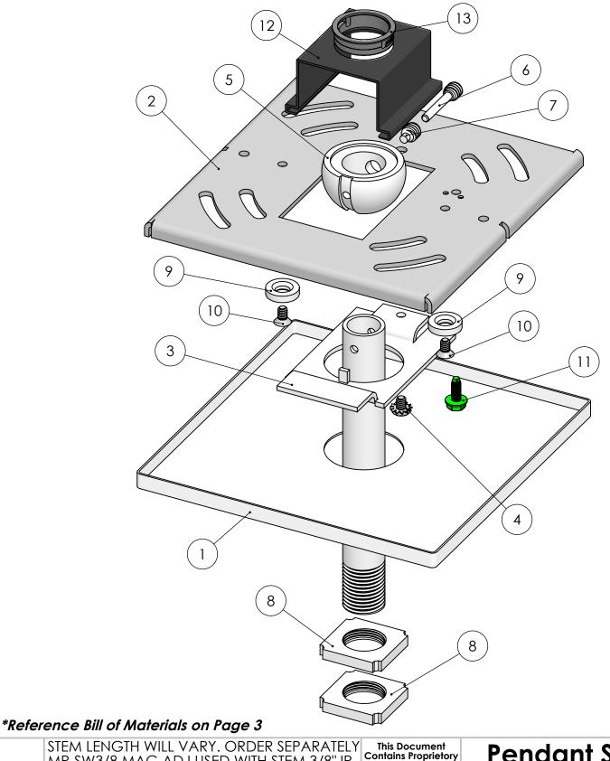
STEM LENGTH WILL VARY. ORDER SEPARATELY MP-SW3/8 MAG ADJ USED WITH STEM 3/8" IP O.D. PH 3/8" IPS .625"-.635" O.D. 18 T.P.I
