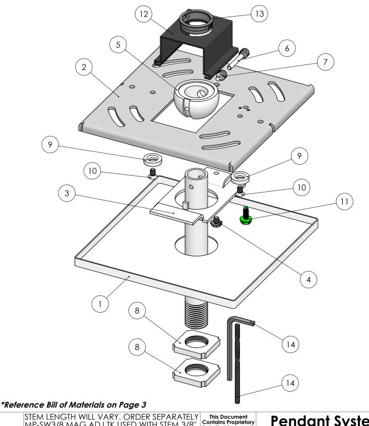
STEM LENGTH WILL VARY. ORDER SEPARATELY MP-SW3/8 MAG ADJ TK USED WITH STEM 3/8" IP O.D. PH 3/8" IPS .625"-.635" O.D. 18 T.P.I
