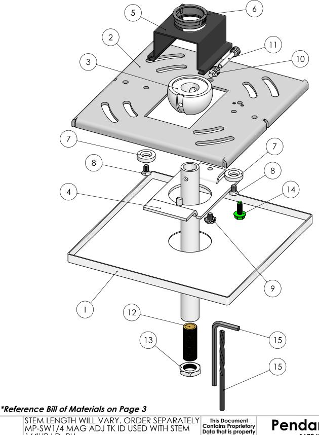
STEM LENGTH WILL VARY. ORDER SEPARATELY MP-SW1/4 MAG ADJ TK ID USED WITH STEM 1/4" IP I.D. PH 1/4" IPS .500"-.510" O.D. 18 T.P.I Add Suffix WHT for White or BK for Black
