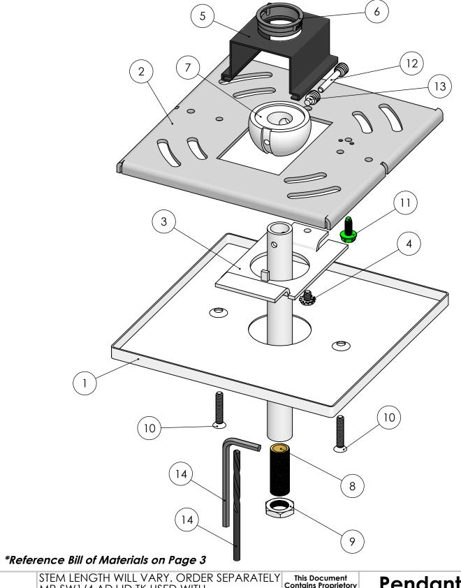
STEM LENGTH WILL VARY. ORDER SEPARATELY MP-SW1/4 ADJ ID TK USED WITH STEM 1/4" IP I.D. PH 1/4" IPS .500"-.510" O.D. 18 T.P.I
