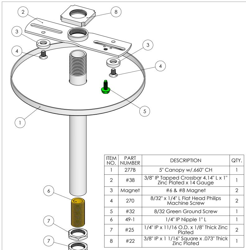
STEM LENGTH WILL VARY. ORDER SEPARATELY C515 MAG ID USED WITH STEM 3/8" IP O.D.-I.D. 3/8" IPS .625"-.635" O.D. 18 T.P.I
