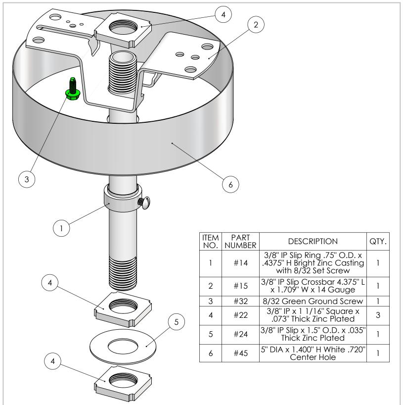
STEM LENGTH WILL VARY. ORDER SEPARATELY C501 TR USED WITH STEM 3/8" IP 3/8" IPS .625"-.635" O.D. 18 T.P.I
