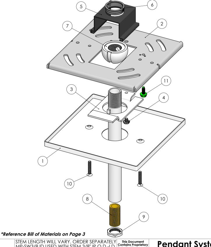
STEM LENGTH WILL VARY. ORDER SEPARATELY MP-SW3/8 ID USED WITH STEM 3/8" IP O.D.-I.D. 3/8" IPS .625"-.635" O.D. 18 T.P.I
