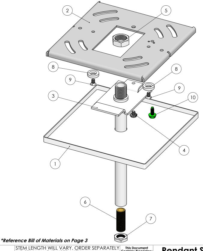
STEM LENGTH WILL VARY. ORDER SEPARATELY MP-ST1/4 MAG ID USED WITH STEM 1/4" IP O.D.-I.D. 1/4" IPS .500"-.510" O.D. 18 T.P.I
