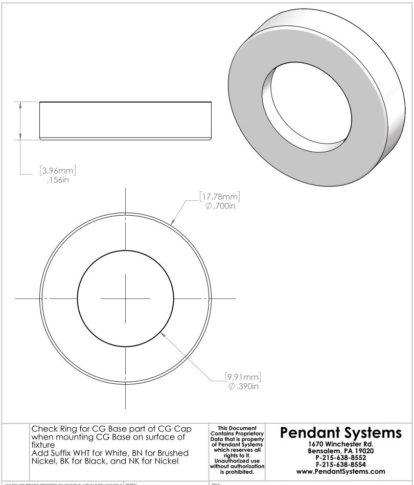
UNLESS OTHERWISE SPECIFIED DIMENSIONS ARE IN BOTH INCHES & MILLIMETERS UNLESS OTHERWISE NOTED TOLERANCES:
