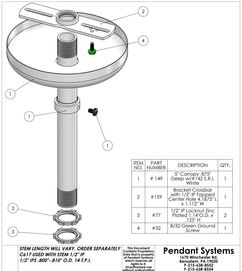
www.PendantSystems.com is prohibited. UNLESS OTHERWISE SPECIFIED DIMENSIONS ARE IN BOTH INCHES & FINISH: MILLIMETERS UNLESS OTHERWISE NOTED TOLERANCES: TITLE: C617 LINEAR: XX= .02" XXX= -.010" ANGULAR: + 1 Degree DO NOT SCALE DRAWING MATERIAL: Part # DEBUR AND BREAK SHARP EDGES REVISION SCALE: NTS SHEET 1 OF 1 DRAWN DATE: 4/7/16 Drawn By: MWR
