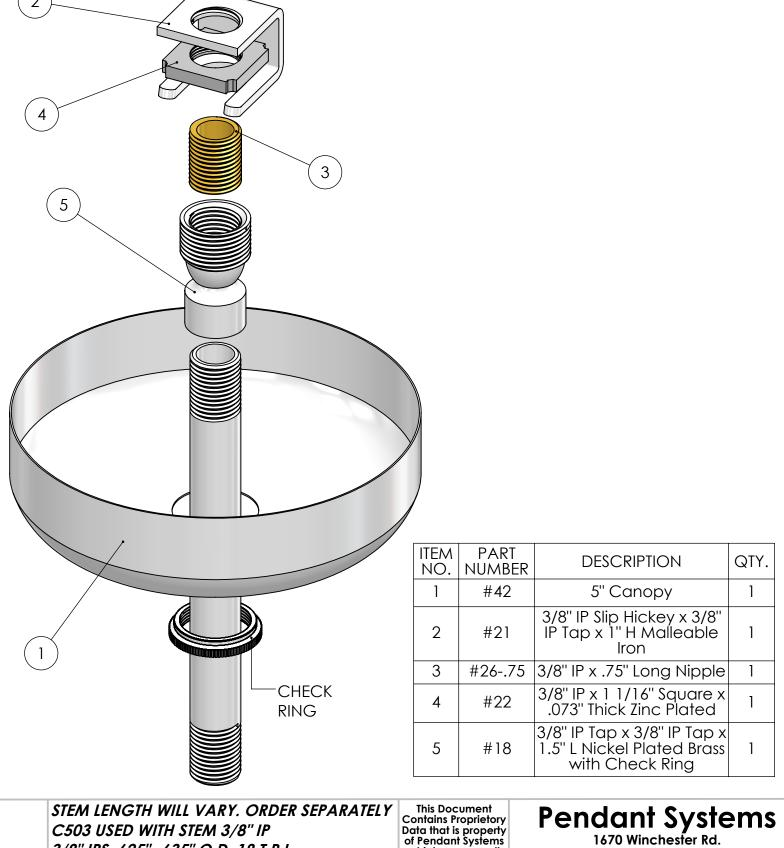
C503 USED WITH STEM 3/8" IP 3/8" IPS .625"-.635" O.D. 18 T.P.I.
