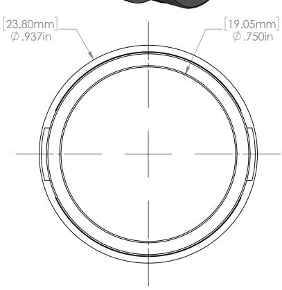
.875" Hole Bushing Black Heyco Part # 2850N .937" W x .750" I.D. x .250" H x .063" Max Pannel Thickness
