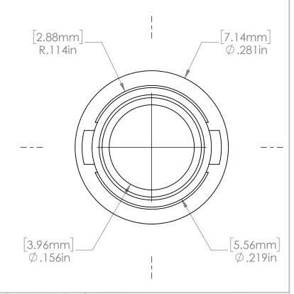
7/32" Hole Plug .25" H Used to plug large side of keyhole for Cross Cables with Half Ball End fittings
