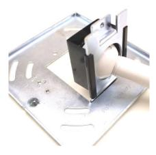
Insert tail end, then shift tapped side on inside of crossbar and fasten with 8/32" screw
