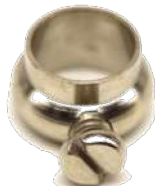
#160- 1/8"IP Slip Ring Nickel Plated W/8/32" Screw .546"W x .322"H (including Flange) x .380"ID .434" Flange
