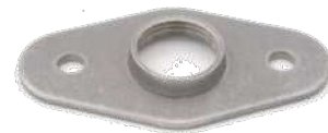
#161 -1/4" IP Tap Center Zinc #162 -3/8" IP Tap Center Zinc 2 5/16" L x 1 1/8" W with 2-#10 Slip Holes Flanges
